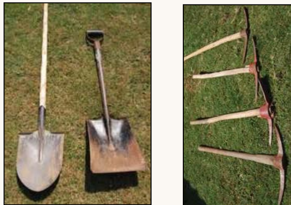
Figure 9: Common tools (picks, spades and shoves) used in salt pan construction. (Photo J. Hinton)
