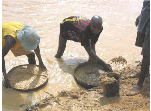
Plate 7: Washing gravel with a shaker at Small Sefadu, 21 st June 2004
