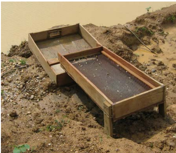
Plate 9: Tool for sorting gravel - The Rocker
